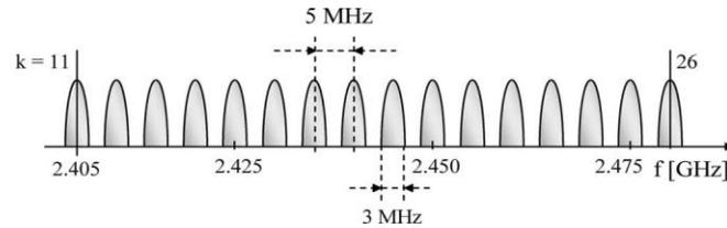
**Fig 3:** Frequency channels of IEEE 802.15.4 inside the ISM band.
