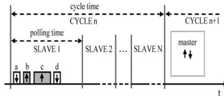
**Fig 6:** Packet exchange between the master and the slave within a polling time.
