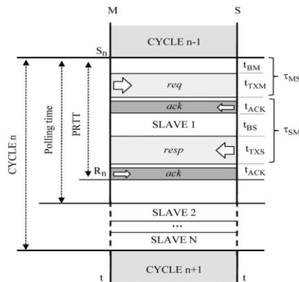
**Fig 5:** Time diagram of the master and slave communication.
