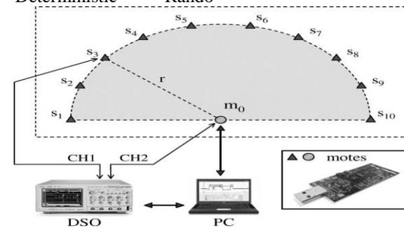
Fig 7: Test bed architecture in the case of ten slaves (N=10)
